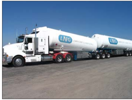
LNG is carried in double-walled, vacuum insulated tankers. Photo courtesy of Chart Inc.
