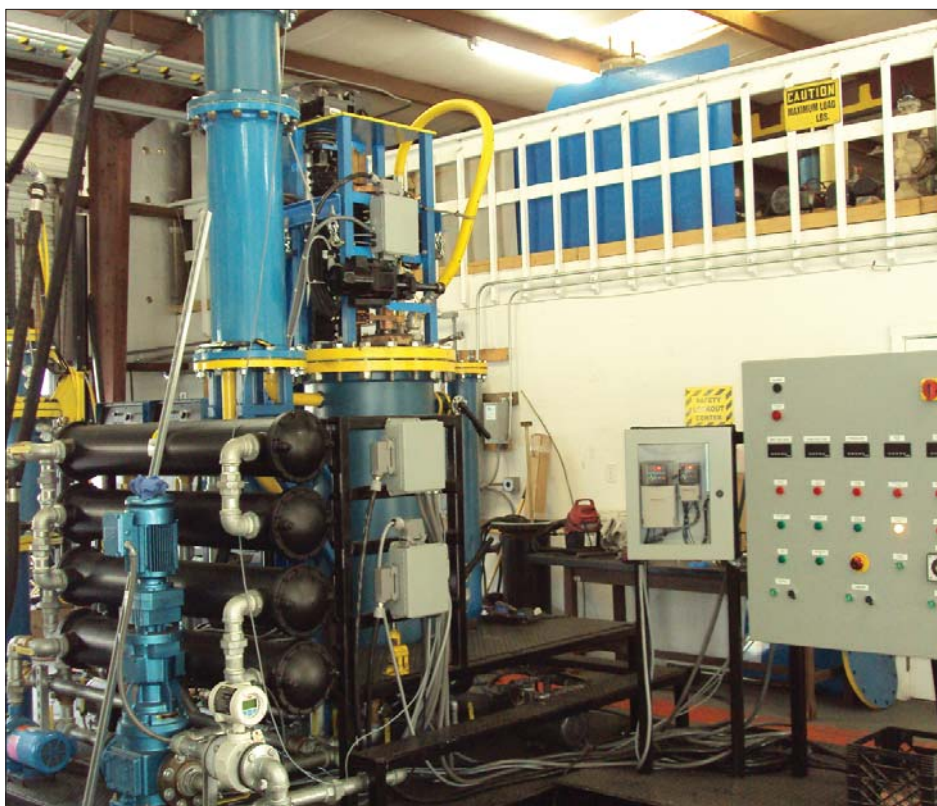
The new MagneGas oil-based waste refinery can produce more than 5,200 cubic feet of clean fuel per hour.
